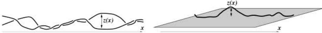
Fig. 1 – Left: bundling of two semiflexible polymers. Right: adsorption of a semiflexible polymer onto a planar substrate.
